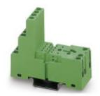
Relay socket PR2-B, for industrial relay REL-IR with 2 or 4 PDT, 1/3-level version, screw connections, connection facility for input/interference suppression modules, for mounting on NS 35/7.5
